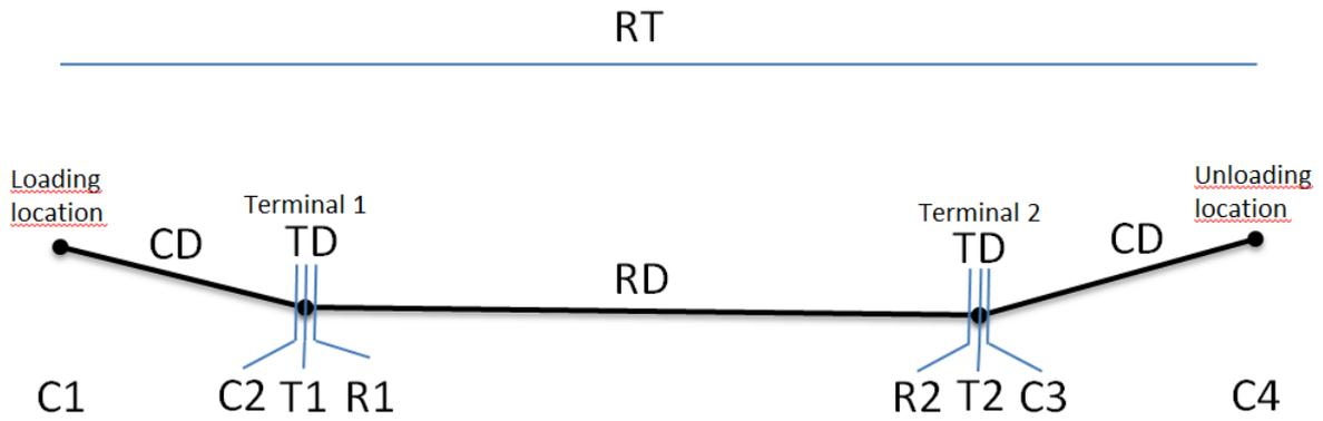
**Figure 4.1: Schematic overview of intermodal corridor with monitoring points**
