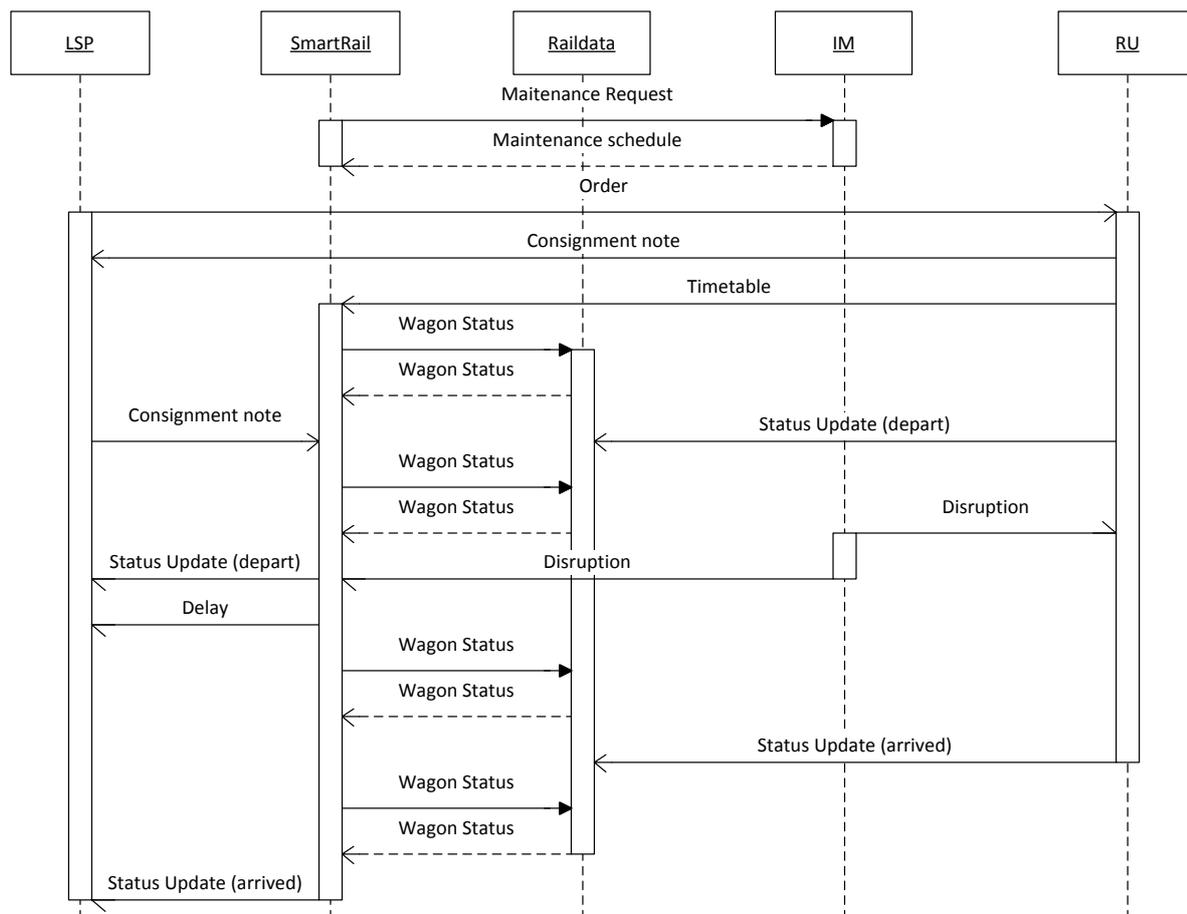
**Figure 3.2: Sequence diagram for handling disruptions**
